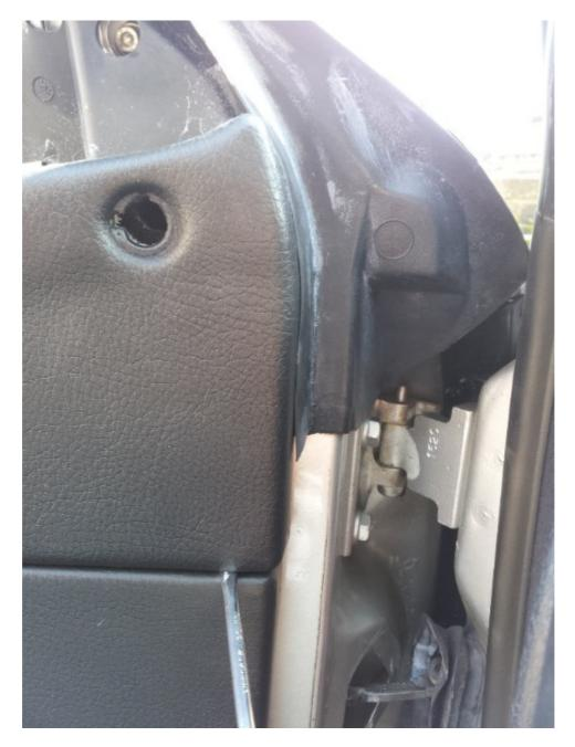
I found by carefully jamming a flat blade screwdriver in the door car as shown above it gives enough of a gap to use another screw driver to replace the rubber seal correctly. Doing it this way also does away with the need of actually taking the door card off.
