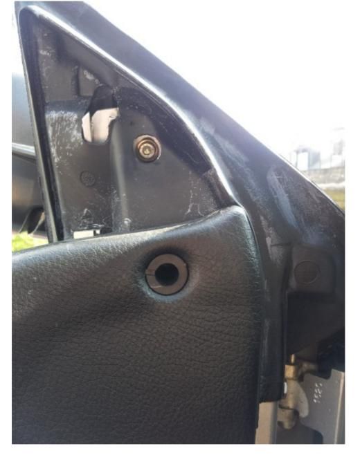
There are 3 screws that you will need to remove to take the whole mirror unit off. 2 of which you can see easily after taking the larger black plastic cover off. The third screw is hidden behind the rubber mirror seal. Carefully pull the mirror seal towards the front of the door and then up to gain access to the remaining screw as shown below.
