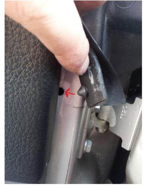
Tighten all the screws up fully and check the rubber seal both inside and out. Also - raise the windows and lower them to make sure the seal is in the correct place. otherwise you'll see "pinching" of the seal. Once you're happy all is as it should be (below) go in for a cuppa.
