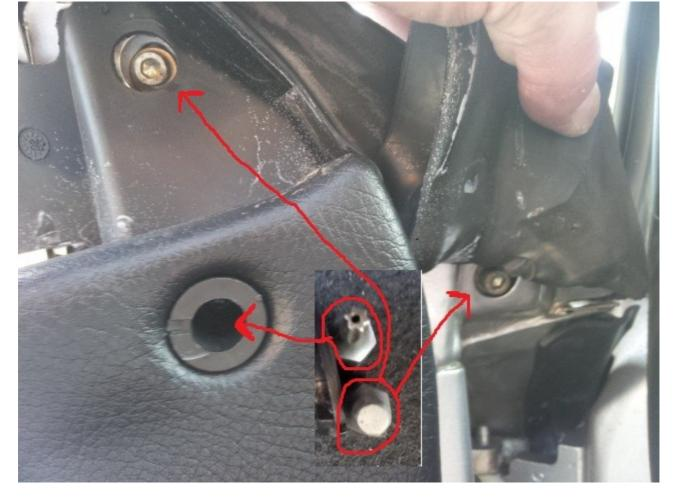
After unscrewing all of the screws, pull the mirror off and balance it somewhere as it will still have the electrical connectors attached.
