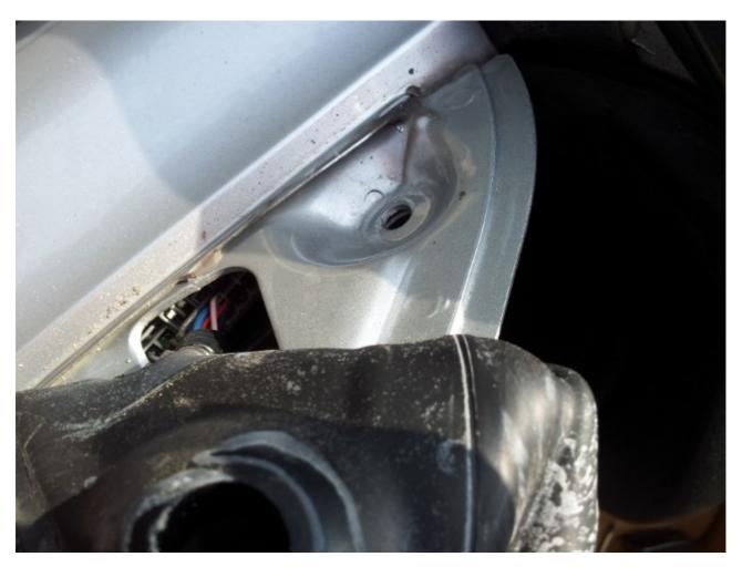
Stick a screwdriver down the hole to free the electrical contact. It can be a bit fiddly but shouldn't take you long. Then pull Ptheidenby: Ct06 Ootupe: Church the rubber seal also. The mirhtipi//www.406boueeedwa.drg
